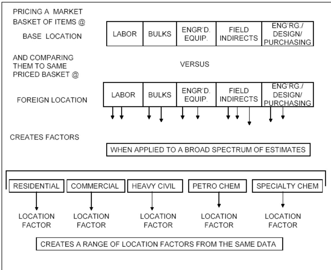
Figure 1 – The Factoring Method Process
